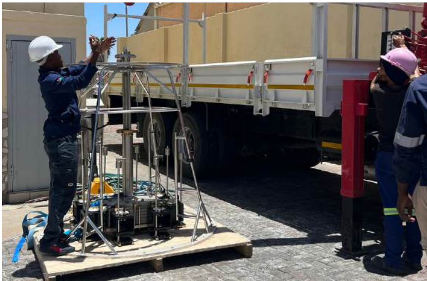
The team boarding the South African vessel MV Good Wind (left) chartered by KFF and equipped with a multi-corer (above), able to dig into the seafloor and extract sediment, keeping layers intact.
